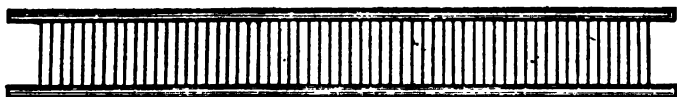
FIG. 7.—THE COMB, OR REED, WHICH BEATS UP THE WEFT-THREAD IN THE LOOM.
